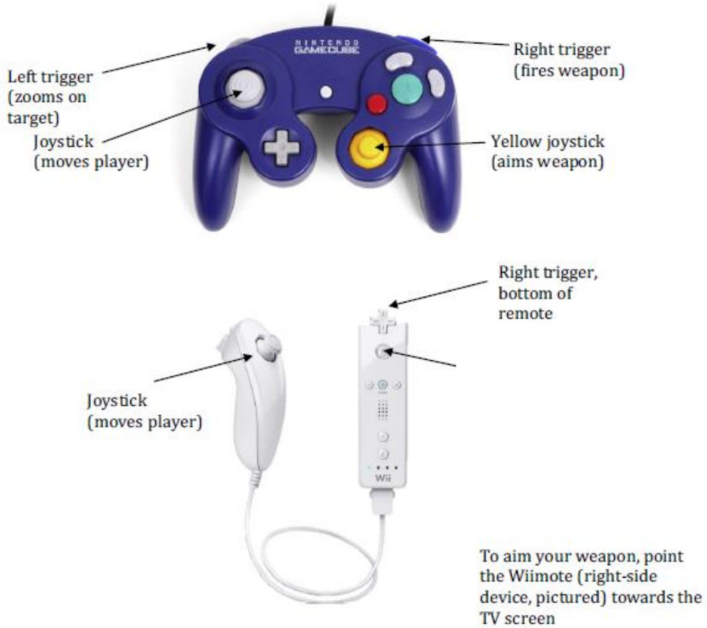
Fig. 1 Different input-output commands to fire a rifle in CoD, comparing traditional GameCube controller (top) and motion-sensor Wiimote (bottom).
