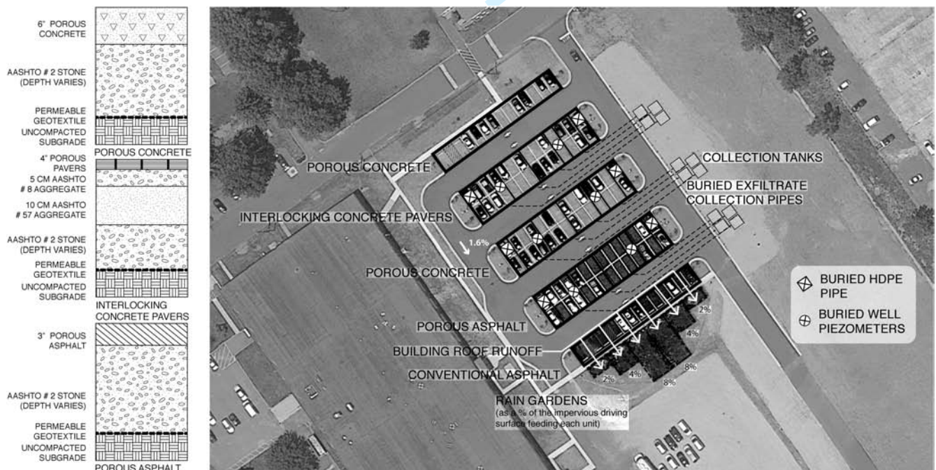
Figure 3. Plan of the permeable pavement parking lot demonstration at the Edison Environmental Center, with vertical cross sections of permeable zones. Portions of the parking rows infiltrate to subgrade soil, whereas others are lined and drain to the collection tanks. Abbreviations: AASHTO, American Association of State Highway and Transportation Officials; CM, centimeters; HDPE, high-density polyethylene.
