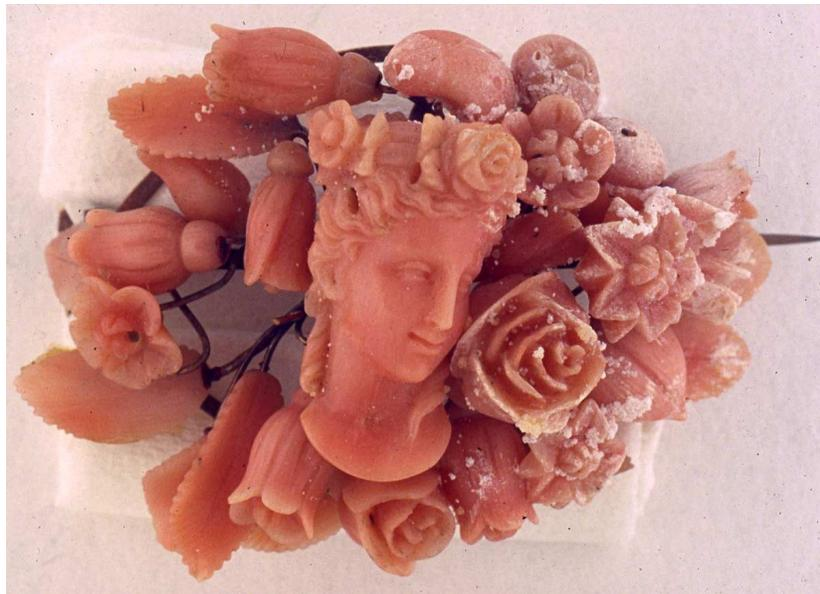
**Figure 7.** A coral brooch and ornaments of cellulose nitrate were stored in an oak barrel for many years causing white corrosion of cellulose acetate-nitrate.<sup>19</sup>
