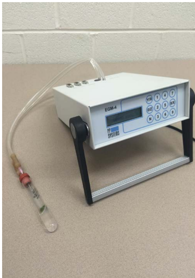
Figure 4. Experimental apparatus of PP Systems EGM-4 Environmental Gas Analyzer and tubing with sample.
