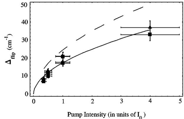
FIG. 10.  $\Delta_{flip}$  vs pump-laser intensity  $I$ ;  $I_0$  corresponds to  $\Omega \sim 20 \text{ cm}^{-1}$ ;  $P_{Ar} = 1 \text{ Torr}$ ; triangles correspond to detunings  $\omega_L > \omega_o$ ; squares correspond to detunings  $\omega_L < \omega_o$ ; solid line is fit to data; dashed line is fit to prediction based on calculated cross sections for collisional transfer. The solid line and the dashed line show the same power-law dependence.
