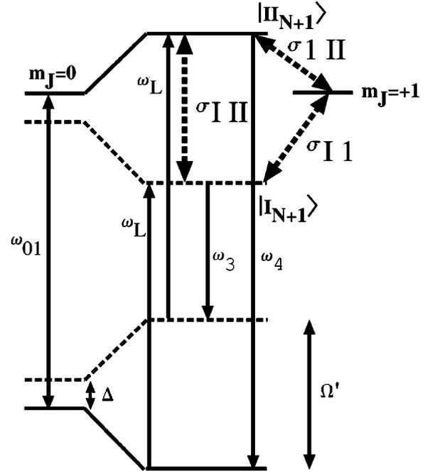
FIG. 2. Dressed states for  $\Delta < 0$ ; the doublets are separated by  $\Omega'$ ;  $\omega_L$  is the laser frequency;  $\omega_3$  and  $\omega_4$  are frequencies for three- and four-photon processes;  $\sigma_{I\ II}$ ,  $\sigma_{I\ 1}$ , and  $\sigma_{I\ 1}$  label cross sections for collisional transfer described in text.
